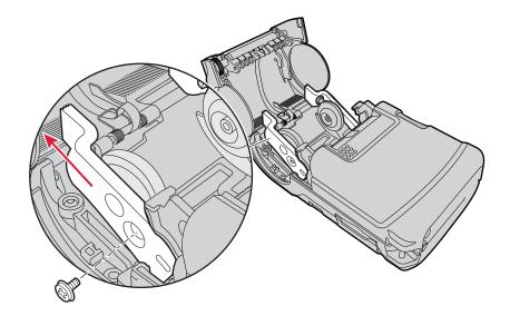
**3** Remove the torsion spring sitting on the media holder and unscrew the media core.
