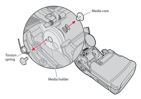
**4** Remove the 19.05 mm (0.75 inch) media core and replace it with the 10.16 mm (0.4 inch) media core.
