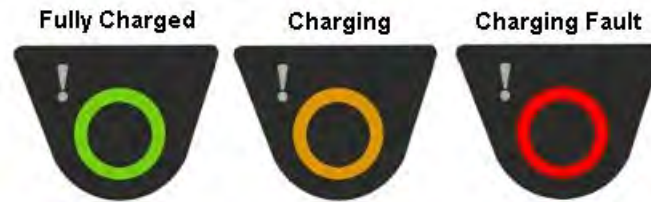
Figure 9: Battery Port Indicators
