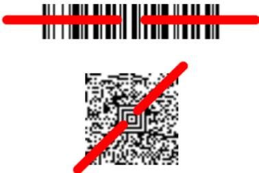
The aiming beam is smaller when the scanner is closer to the code and larger when it is farther from the code. Hold the scanner close to smaller bar codes, and farther away from large bar codes to get a proper read.
