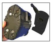
Facing the printer, move the locking lever to the "locked" position (from the left to the right) until it "clicks" into the "locked" position.
